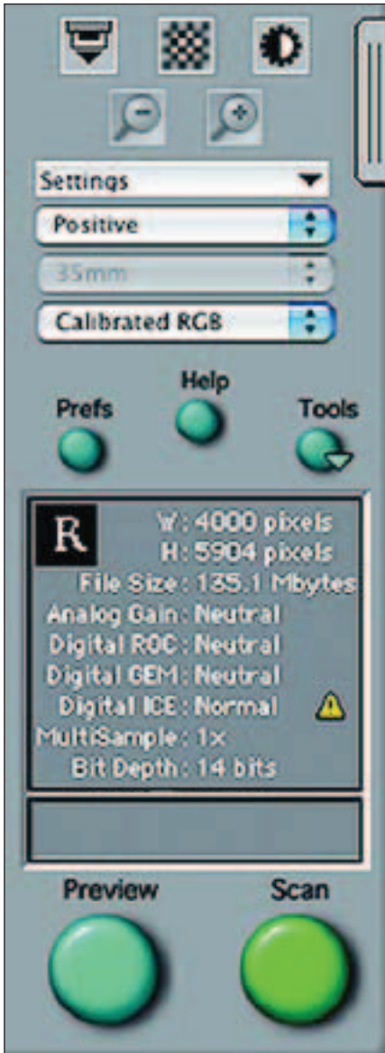
FIGURE 2-3. NIKON SCAN CONSOLE. Preview the scanner settings summarized in the Console window before scanning.
